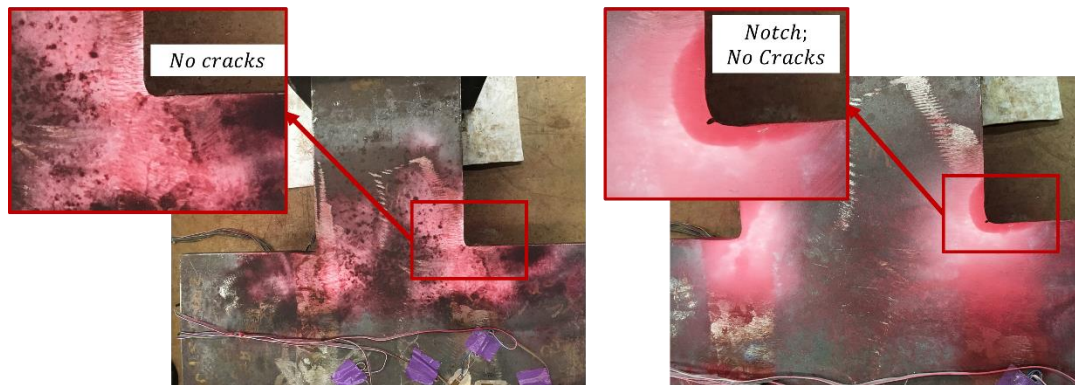
Figure 52. Dye penetrant progression: a) 6 million cycles; b) 10 million cycles
