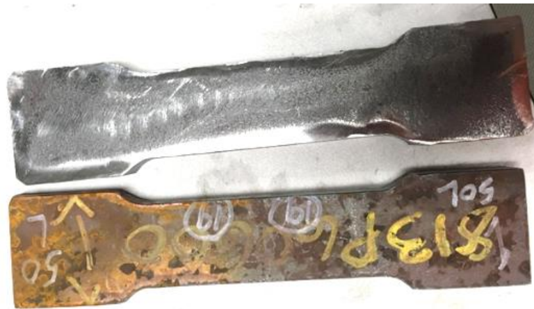
Figure 31. Corroded (bottom) and uncorroded (top) steel surfaces
